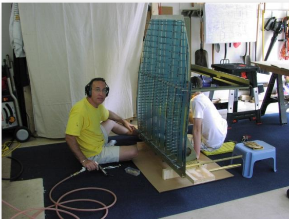
1. Riveting the bottom center section skin to the ribs with my son. I had already riveted the ribs to one half of the spar box.
